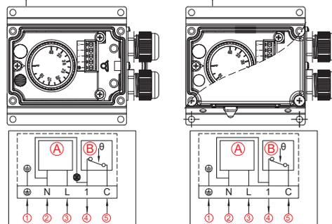
(A) Electronic circuit (B) Relay Max 16A 240V res.
